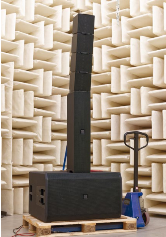
MAILA array above the subwoofer The lashing strap visible at the back only served to secure the system during the measurement in the inclined set-up
